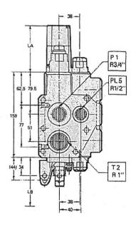
The measurements given above apply to the valve housing and spool control positions
