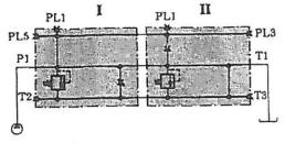
Single-pump operation with carry-over connection, type K2.
