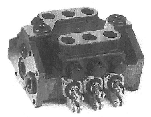
The RM 310 is a modular parallel monoblock valve with 1 - 4 sections. It is designed for a maximum working pressure of 225 bar and for a recomended flow range of 40 - 120 l/min.
