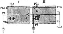
Two-pump operation with carry-over connection, type K5.
